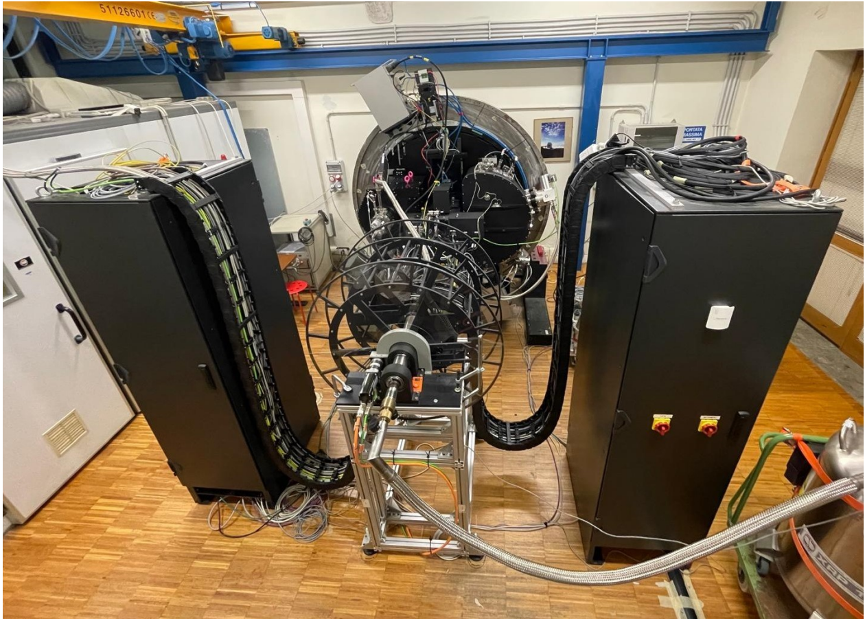
Figure 1. The SOXS instrument fully assembled in the integration hall of the Padova Astronomical Observatory. It is mounted on the NTT simulator flange, providing the same interfaces of the real telescope at the Nasmyth focus. The instrument can be rotated and tested in all gravity conditions. The co-rotator structure is visible in the center with two lateral cable-wraps which safely support the cables during the rotation. The two black cabinets on the left and right host most of the control electronics. The only missing part in this picture is the Nasmyth platform, which has already been shipped and installed in Chile.
