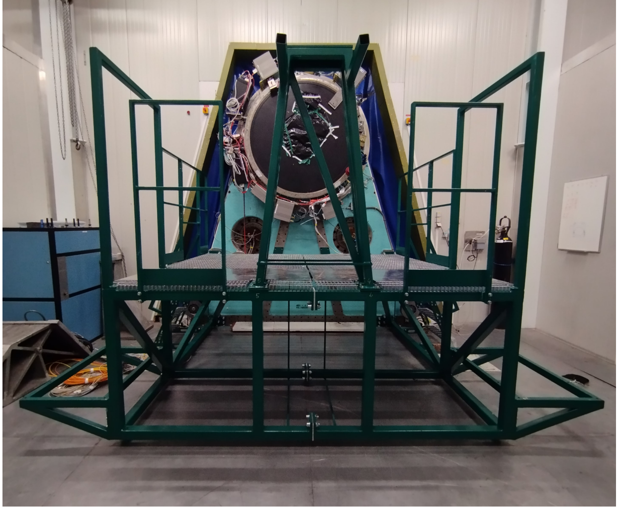
Figure 9. The SOXS platform fully assembled and installed at the NTT in the La Silla Observatory. It will support the co-rotator structure as well as the two electronic cabinets.
