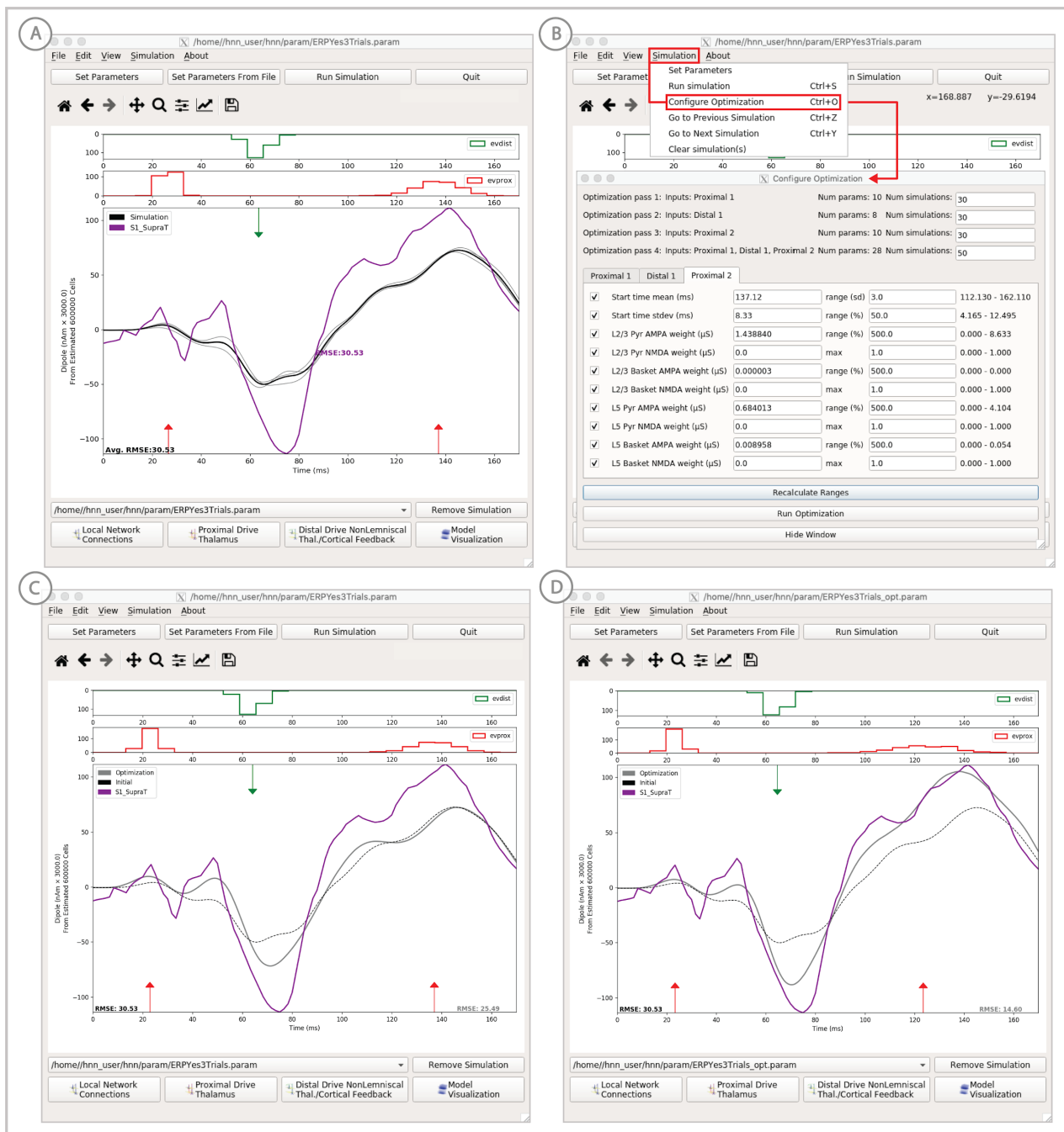
Figure 10: Example of the ERP parameter optimization procedure for a suprathreshold tactile evoked response. (A) Source localized SI data from a suprathreshold tactile evoked response (100% detection; purple) is shown overlaid with the corresponding HNN evoked response (black) using the threshold level evoked response parameter set detailed in Figure 4, as in initial parameter set. The RMSE between the data and the model is initially high at 30.53. (B) To improve the fit to the data, a serial procedure for optimizing the strengths of the proximal and distal drive input generating the evoked response can be run, by choosing the “Configure Optimization” option through the “Simulation” pull down menu. A dialog box allows users to choose and set a range over free optimization parameters, see text for details. (C) The GUI displays an intermediate fit after the first optimization step, specific to the first proximal drive. (D) The final fit is displayed once the optimization is complete. Here, the simulation from the optimized parameter set for the suprathreshold evoked response is shown in gray with an improved RMSE of 14.60 compared to 30.53 for the initial model. See Figure 10 Supplementary Figure 1 and 2 for further description of the optimization routine and a parameter sensitivity analysis.
