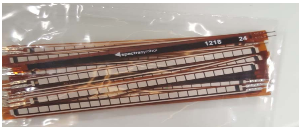
Fig. 8 Flex sensors used in determining the deflection angle. (colour online only)
