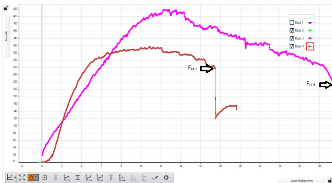
Fig. 13 Force (N) vs. deflection ( \Delta X , mm) for a field grown Acacia totilis (brown) and a nursery grown one (violet). (Field Acacia: S=2.00 N/mm and F_{crit} = 260 N. Nursery Acacia: Slope= 1.71 N/mm and F_{crit}=210 N). (colour in print)
