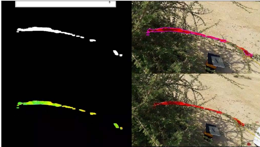
Fig. 17 A snapshot of the video illustrating the results of IPT. The lower right panel shows the branch under study covered in red tip while subjected to a bending force. The right upper panel shows the branch highlighted. The left panels show the branch after the color was converted to HSV and a red filter was applied to produce a binary image. The red pix was changed to white and the rest of pixs were changed to black. To watch the video, follow the link ( https://youtu.be/TSjYAzsahTk ). (colour in print)
