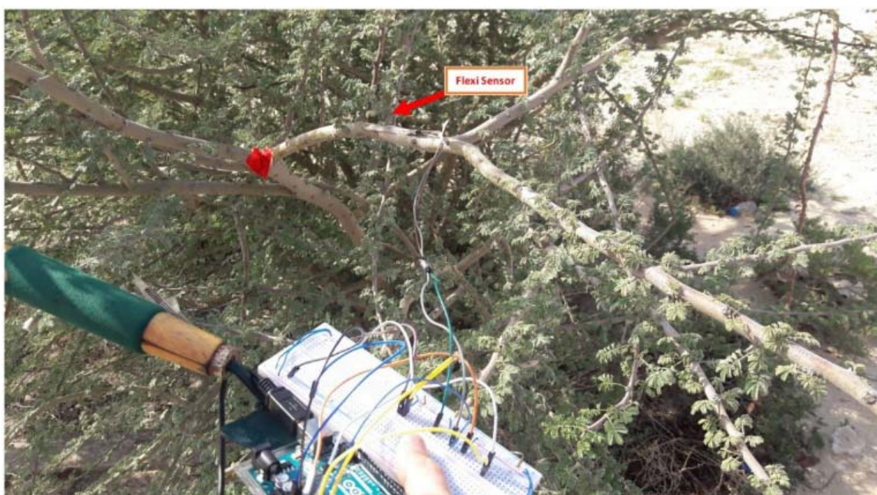
Fig. 10. Deflection angle measurement setup. (colour in print)
