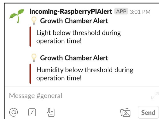
Figure 3: A snapshot of what an incoming alert from the GMpi looks like on Slack. This will alert all members of this workspace that the growth chamber has fallen out of the specified range for both light and humidity.
