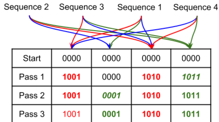
Figure 3. An example set of insertions causing saturation of some of the key-value association in the miBF. Sequences 1 and 2 can still be reliably be used for their key-value pairings, but sequences 3 and 4 will return completely saturated IDs such that they cannot be trusted to return all possible associated IDs to that sequence if it is queried.
