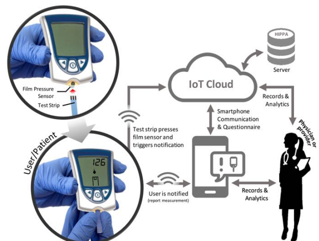
Fig. 1. Schematic of the overall functionality of the GlucoPush add-on system. Insertion of the test strip in the glucometer compresses the installed film pressure sensor which then triggers a notification for measurement storage in secure cloud via a smartphone.
