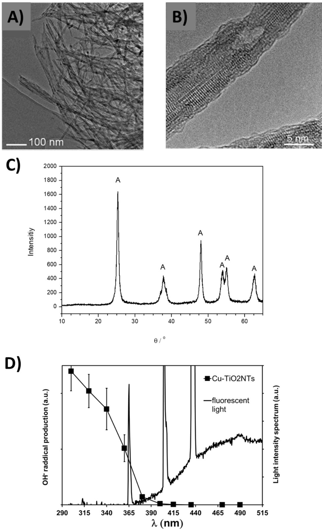
284 **Figure 1. Structure and photocatalytic activity of Cu<sup>2+</sup>-doped TiO<sub>2</sub> nanotubes (Cu-TiO<sub>2</sub>NTs) excited at different wavelengths. A) and B) TEM images of the nanotubes**
