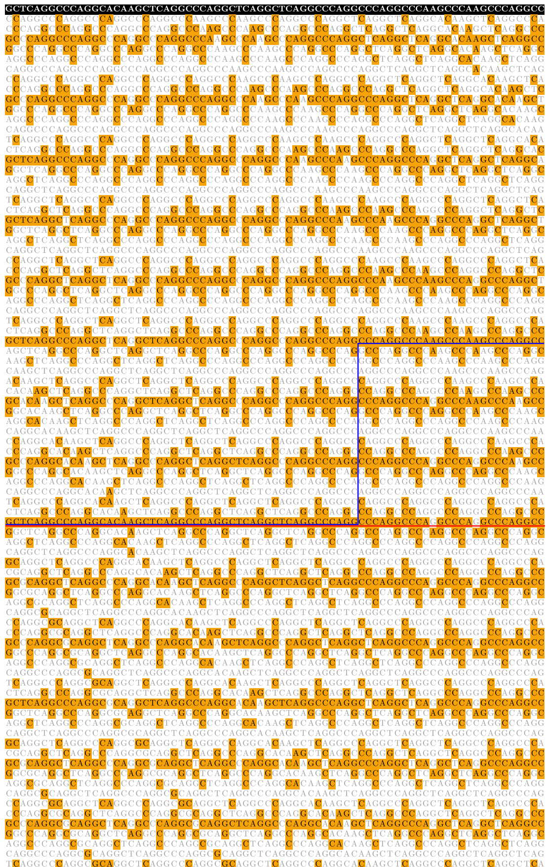
Fig. S8. Illustration of the match matrix. The top line with white letters on a black ground specifies the nucleotide sequence of a read. Other lines represent nucleotide sequences of the reference genome shifted by one nucleotide with respect to the previous (upper) line. Matched nucleotides are highlighted with a yellow colour which creates the match matrix (yellow = True, white = False). Two read alignments are shown. The naive way to align a read with two mismatched nucleotides is shown as a red straight line. The path with one deletion, which takes into account the highly mutative nature of STRs/QTRs, is shown with a blue line.
