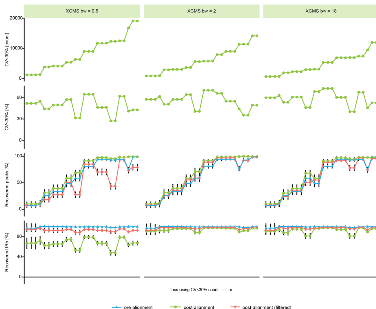
Figure 5. A dataset consisting of 9 replicate injections was processed via XCMS using different values for the maximum allowed peak width (MPW) parameter and the bandwidth (bw) parameter, leading to a total of 78 non-targeted data pre-processing experiments. Four different quality metrics including the number of features with CV < 30%, the proportion of features with CV < 30%, and the proportion of recovered benchmark peaks and isotopologue ratio biases (IRb) (pre-alignment, post-alignment, and post-filtering (only features without missing values and with CV < 30%)) were then plotted (sorted by increasing number of features with CV < 30%).
