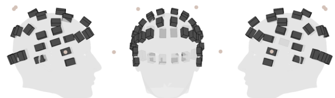
Fig. 3. Position of each of the OPMs (black cuboids) and retroreflective markers (orange circles) in the auditory experiment. The participant's head is represented by the grey mesh.
