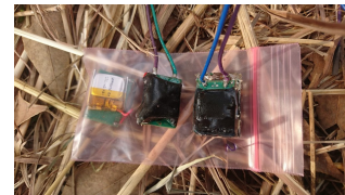
Figure A.8: Top: Landscape showing habitat in which trials were carried out; Bottom: Prototype loggers (two with epoxy) used in trials
