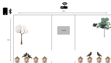
Figure A.9: Layout of the starling aviary for the field trial. The feeding station is in the centre of the aviary, with a stationary logger attached. Nest boxes are arranged along one side of the aviary, with a camera trap placed in front of each. Blue squares represent the stationary loggers while yellow squares represent the mobile loggers. A gateway was placed adjacent to the feeding station but on the outside of the aviary to allow easy access and ensure that mobile loggers would be downloaded. In addition, data could be read and logger settings adjusted through the use of the mobile application.
