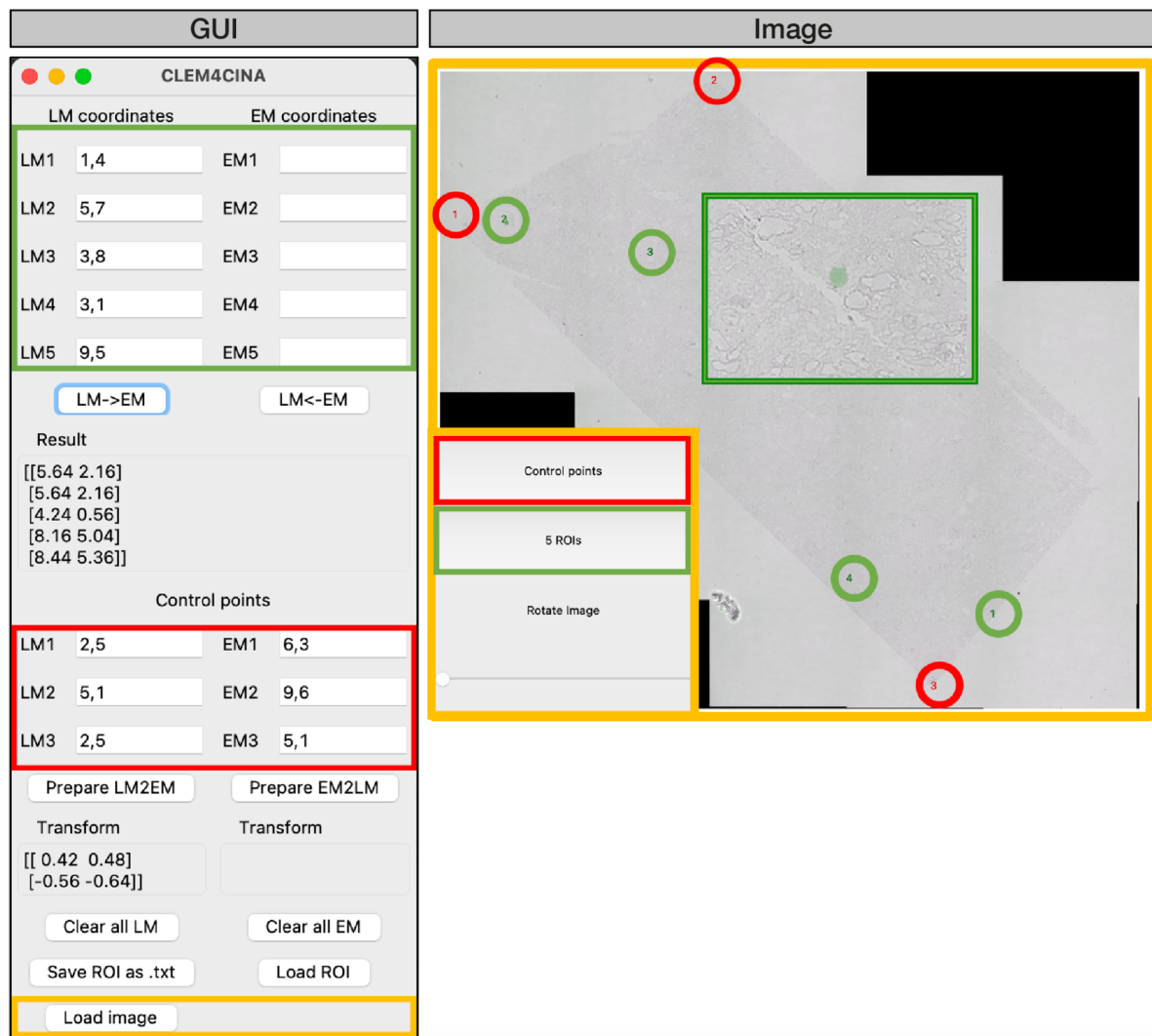
Supplementary Figure 8. The GUI for the CLEM4CINA program. An image is loaded into the GUI (orange frame GUI) that will then be displayed in a top view window (orange frame, Image). Two button widgets (inset, Image) prompt the user to click on three control points (red frame) and five ROIs (green frame) in the loaded image. Examples of selected points are displayed and numbered in the image in the corresponding colours. The coordinates are automatically entered into the green and red frames of the main GUI. The mouse wheel can be used to zoom into the image (green frame, left). A slider on the widget panel under 'Rotate Image' (inset, Image) allows the user to rotate the displayed image.
