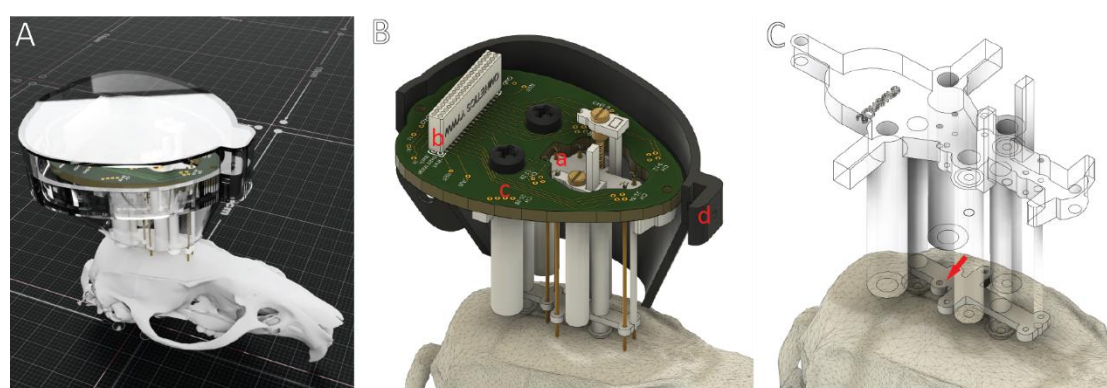
Figure 1: Overview of the TD drive. A. Rendering of a TD drive with protective cap. B. Rendering with inner parts shown. The TD drive features (a) multiple, parametrically adjustable recording locations for fixed and moveable electrode wires, an EIB with (b) a high-density Omnetics connector compatible to common tethered and wireless data acquisition systems and (c) an intuitive channel mapping optimized for recordings with Intan/Open Ephys systems and (d) a cap to protect the implant during tethered recordings and when no headstage is connected. C. A guide stencil on the bottom of the TD drive facilitates placement of guide cannulas and serves as a redundant verification of implant locations during surgery.
