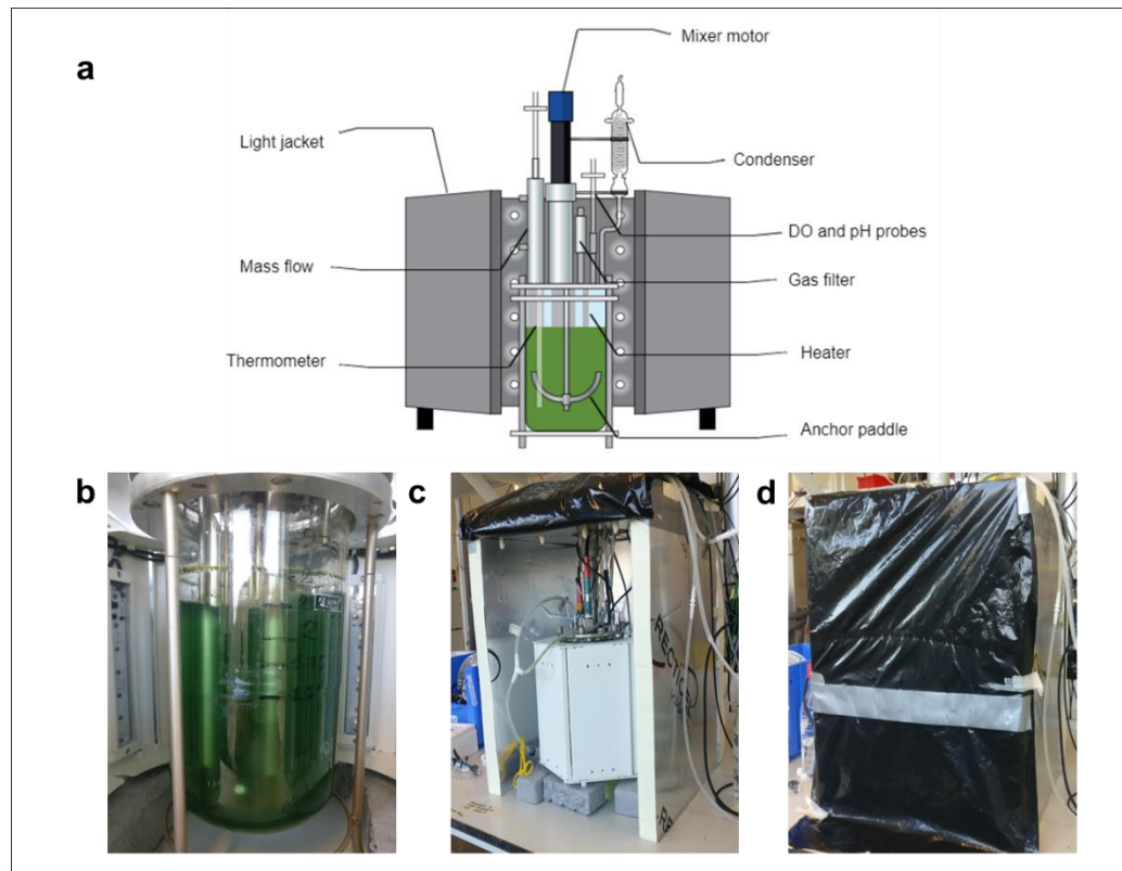
Figure 1 a. Photobioreactor set up with a light jacket surrounding it. The temperature was kept at 35°C and argon was injected in the reactor. The incoming gas was controlled by a mass flow controller, while the off-gas was cooled by a condenser and filtered with a cotton filter before it was sent to the off-gas analyzer. DO, temperature, and pH were continuously measured in all set-ups. For the chemostat regime, influent and effluent flows were regulated by pumps. Acid and base were dosed to maintain the pH at 7. b. Picture of the reactor the a and light jacket. c. Picture of the PIR-boards hood built to avoid the influences of external light and temperature. d. PIR-boards hood had a black plastic cover that enabled access and hinder the entry of external light.
