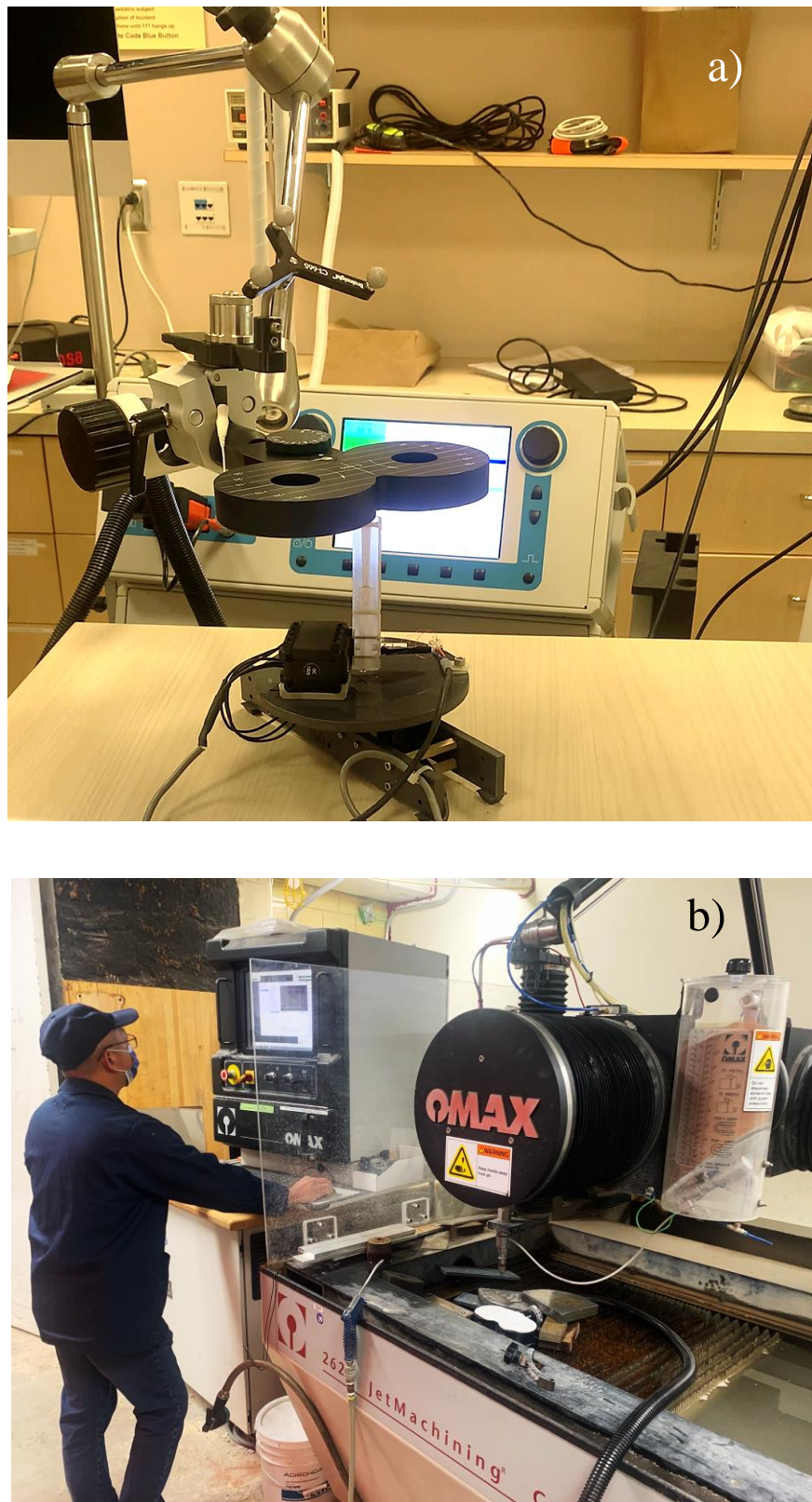
Fig. 7. a) NKI E-field triangular probe. b) Waterjet dissection of the MagVenture C-B60 Coil.
