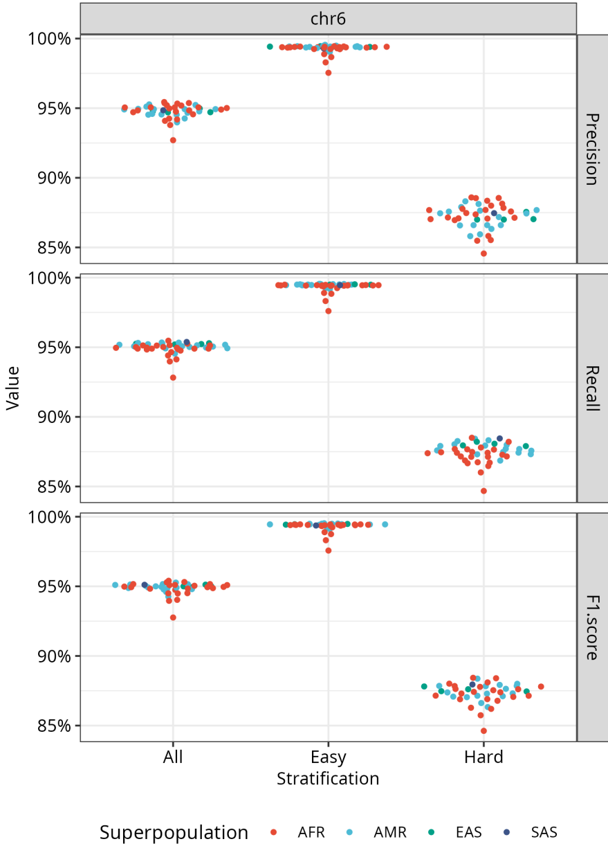
Fig. B4: Precision, recall, and F1-score of small variants in the H. sapiens chromosome 6 pangenome graph relative to HiFi-DeepVariant calls. Comparisons are made whole-chromosome and then stratified by the GIAB (v.3.0) genomic context. The 44 samples evaluated are colored by superpopulation. AFR = African, AMR = Ad Mixed American, EAS = East Asian, SAS = South Asian.
