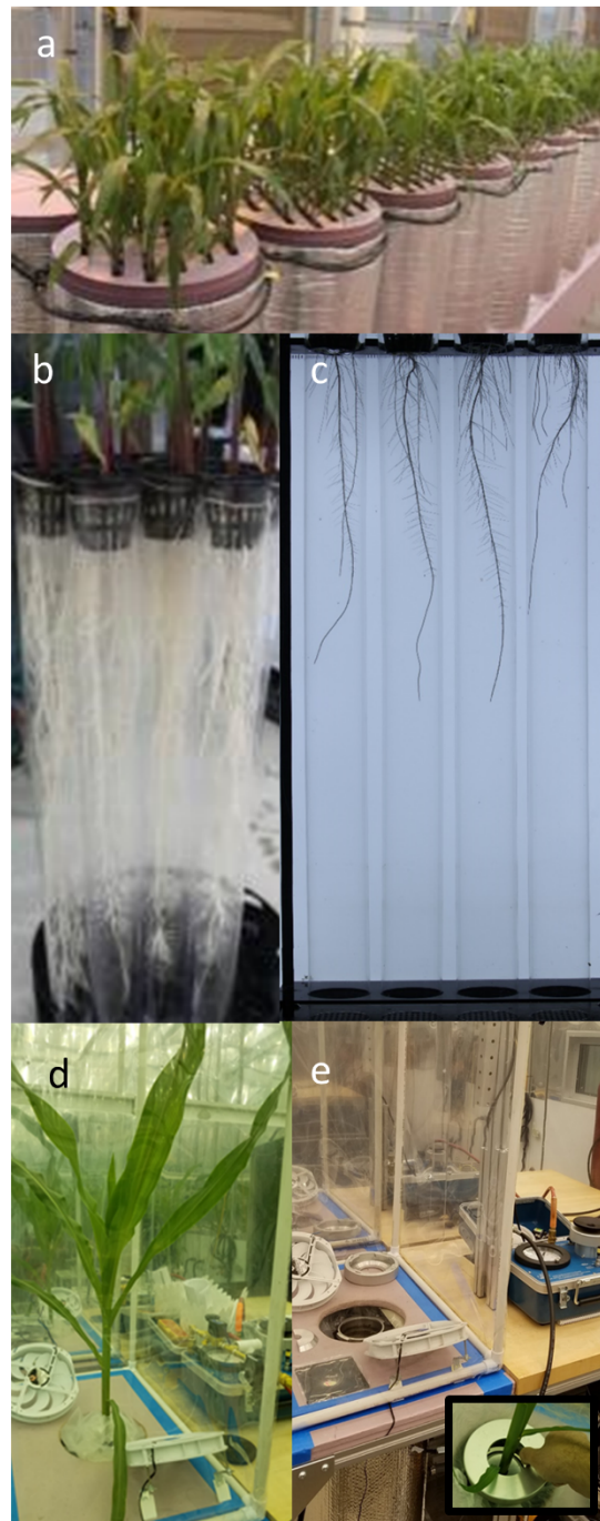
Figure 2. Temperature-controlled root phenomics platforms: 1) hydroponic root growth platform showing the temperature-controlled root growth platform module with growth tanks containing maize plants (a), a rack with individual growth tubes (b), and a raw image of root systems captured during root growth experiments (c), and 2) pressure chamber with root temperature control (d,e).
