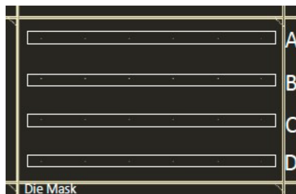
Figure 2. Arrangement of constrictions on a silicon device.
