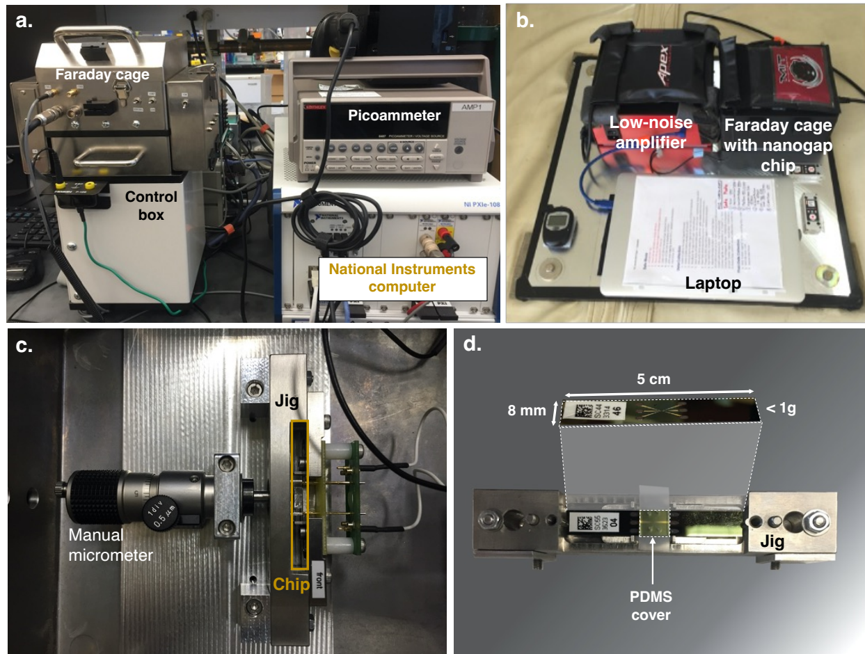
Fig. 3. ELIE Instrument Prototype. a , Benchtop Osaka University Nanogap System used for the analysis of amino acids in Ohshiro et al. 2014. b , Current system consisting of a laptop controlling the low-noise amplifier that, in turn, supplies and controls voltage to and within a Faraday cage that encloses c , a manual micrometer and jig structure holding the d , nanogap chip.
