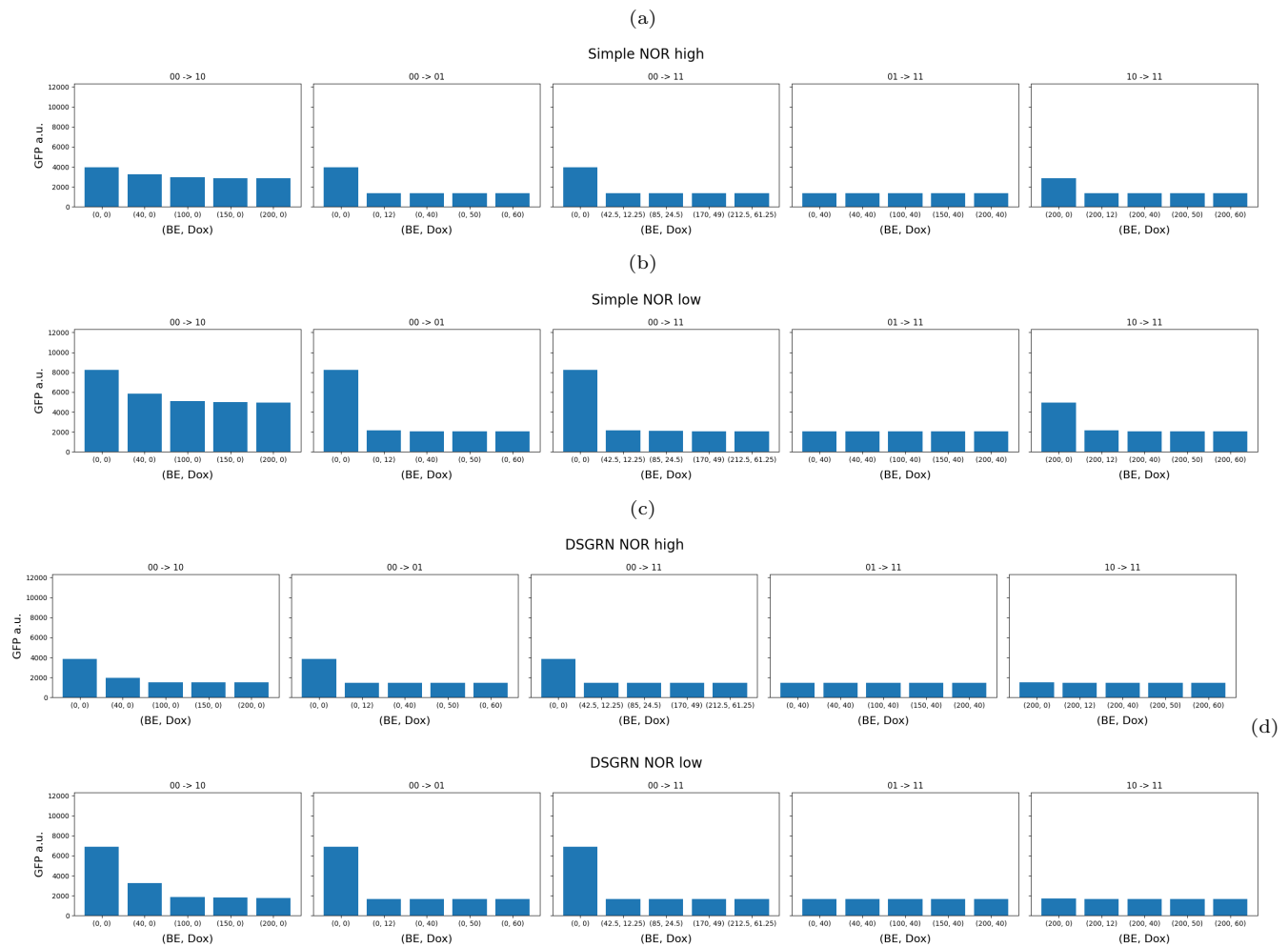
Fig. 15. Predicted steady-state values of the geometric mean of the flow cytometry distribution of GFP a.u. using estimated Hill function parameter values for: (a) Simple NOR/CDM low design, (b) Simple NOR/CDM low design, (c) DSGRN NOR/CDM high design, and (d) DSGRN NOR/CDM low design. An OFF circuit state corresponds to approximately 1500-2000 a.u.; robust ON circuit states occur at about 8000 a.u. and up, and weak ON states occur at about 4000 a.u. Columns 1-3 (transitions 00 \rightarrow 10 , 00 \rightarrow 01 , 00 \rightarrow 11 ): The left-most bar in each bar graph should be ON. All other bars should be OFF. Columns 4-5 (transitions 01 \rightarrow 11 , 10 \rightarrow 11 ): All bars should be OFF.
