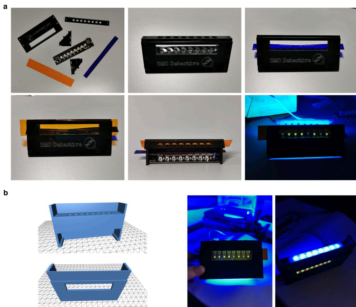
Figure S3: Comparison of acrylic and 3D printed GMO Detective device. a) Acrylic version of the GMO Detective device. b) 3D printed version designed in openSCAD to accommodate the same filters and PCB used in the original device. All editable files available in https://github.com/MakerLabCRI/GMODetective-Detector/blob/main/3D%20Model/STL/GMO detective3D.stl
