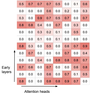
Figure 3: There are two types of heads emerged in Infini-attention after training: specialized heads with gating score near 0 or 1 and mixer heads with score close to 0.5. The specialized heads either process contextual information via the local attention mechanism or retrieve from the compressive memory whereas the mixer heads aggregate both current contextual information and long-term memory content together into single output.
