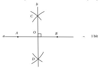
*Remark.* If the first circle was drawn with an arbitrary radius but the second circle was made by a radius unequal to the first radius, this implies 1 bit of ratio equivalent to a ratio other than 1. This setting implies the extra bit of side because breaks the symmetry of the geometrical shape. Therefor we have 2 bits and expect that the transversal line between intersection points cuts the line AB to produce two segments equivalent to 2 bits. We discuss it in detail in the next example.
