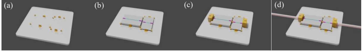
Figure 6 Schematics of the process flow for the chiplet integration. The components are not in scale. (1) The fixers and clamps are printed on a silica substrate. Optional adhesives like crystalbond wax or UV glue can be applied. (b) The chiplets are placed with the help of fixers. (c) Reflectors and the funnels are on-chip-printed. (d) I/O optical fibers are inserted and guided by the funnel structures.
