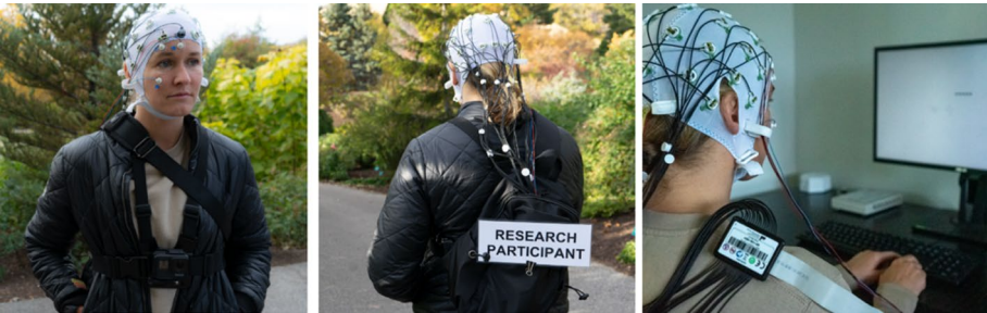
Figure 3. Left and middle: participant walking setup. See Supplemental Materials for GoPro camera data. Right: attention network task and EEG recording setup in the laboratory. Informed consent was obtained from the pictured participant for these images to be included.
