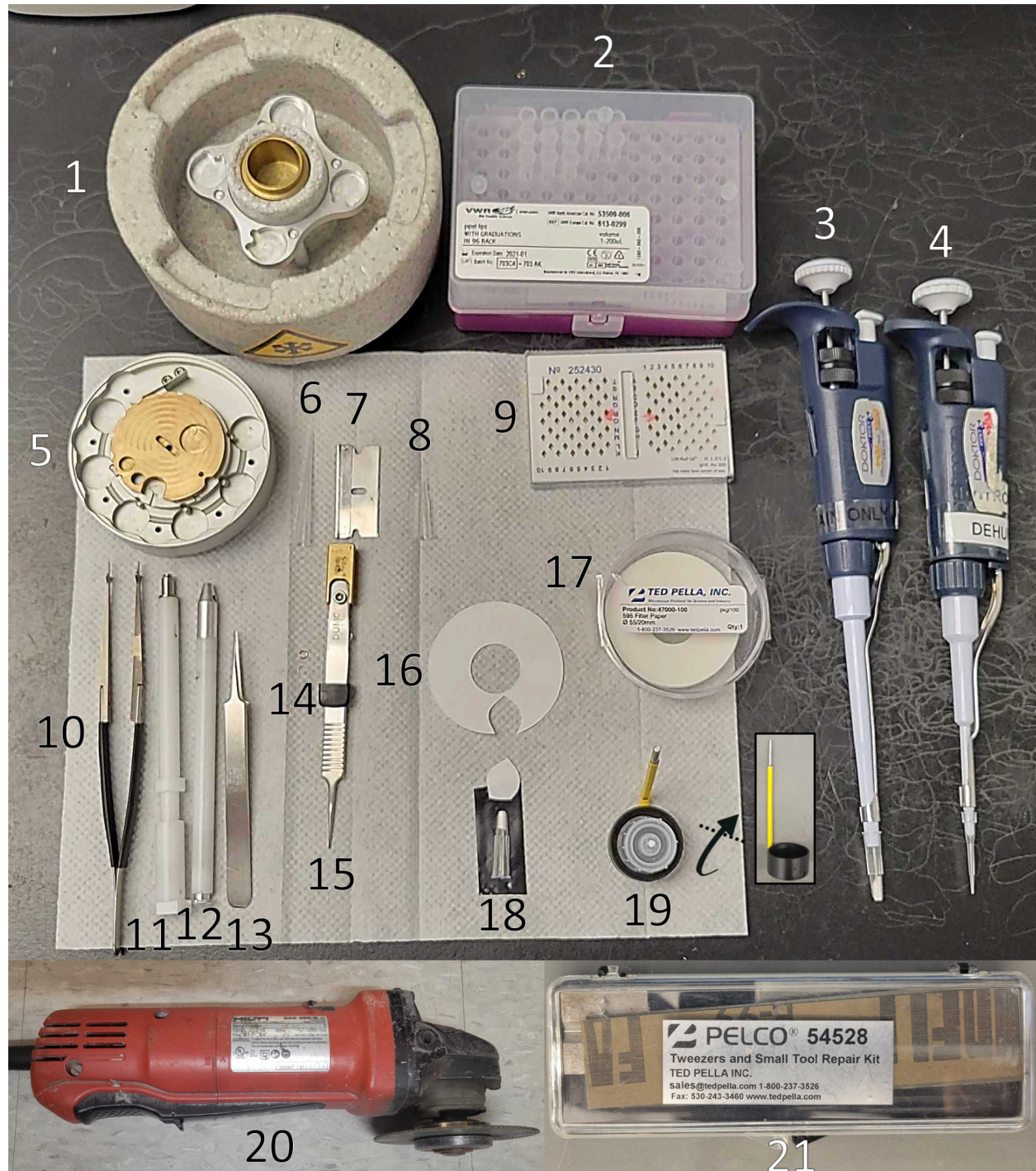
Supplementary Figure 10 | Items recommended for preparing CryoCycle blotting methods along with numbers corresponding to Supplementary Protocol 1. Note: CryoCycle modified pipette tips may be created with any pipette tip that has an inner diameter smaller than 3 mm; A 200 \mu L pipette tip is shown here. 1,000 \mu L and 200 \mu L pipette tips are shown in Figure 1 . Note: an autogrid clipping station (item #5) is not required; Room temperature grids can be clipped on a flat surface without a clipping station.
