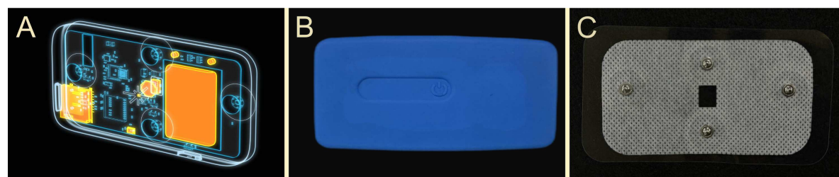
Figure 2. Multi-modal recording hardware. A: X-Ray diagram of the device and its components. B: Front of the device. C: Front of the electrode patch that clips to the back of the device.
