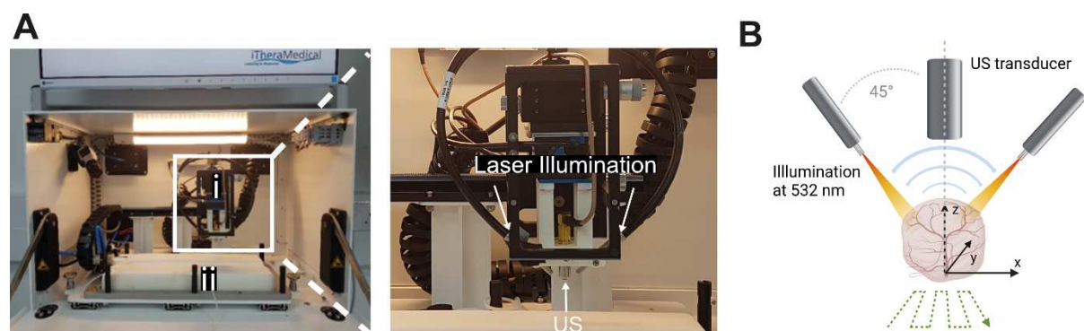
Figure 1: Overview of the photoacoustic mesoscopy system. A) Photograph of the system. (i) denotes the scan head and (ii) the heated mouse bed. The scan head is enlarged in the second photograph. Top arrows are pointing on the two illumination fibres, whilst the bottom arrow points on the ultrasound (US) transducer. B) Schematic illustrating the functioning of the system. Created with Biorender.
