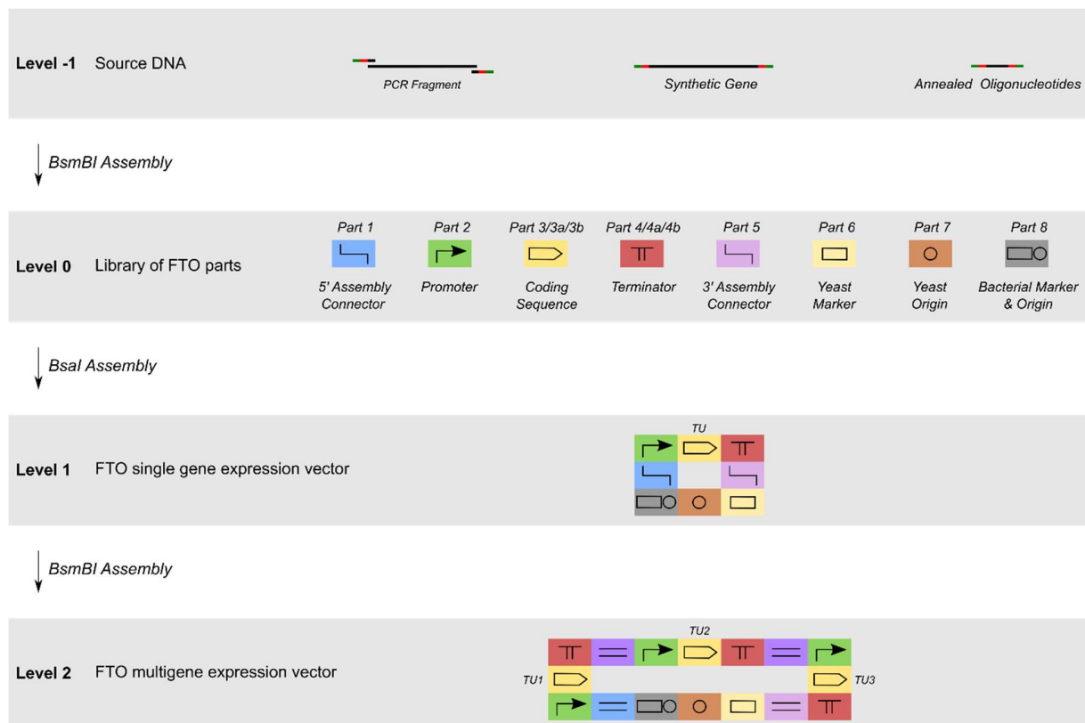
Figure 8. The modular cloning or MoClo principle. In a first phase, source DNA, such as PCR fragments, synthetic genes or annealed oligonucleotides are flanked with the proper Type IIS restriction sites and 4 nt overhangs, which are then accommodated in a Level 0 entry vector through BsmBI digest and T4 DNA ligation. Then, selected Level 0 vectors are assembled into a Level 1 expression vector by means of a BsaI digest and T4 DNA ligation. Finally, the system allows the assembly of multiple transcription units (promoter, CDS, terminator) from the individual Level 1 vectors, into a higher order Level 2 vector, in case the assembly connector sequences were properly selected during the assembly of the Level 1 vectors. Assembled assembly connectors are depicted with two horizontal lines and different shades of blue and purple. Note that the Part 3 Coding Sequence can be split up in a Part 3a and Part 3b Coding Sequence, to allow additional modularity. Likewise, the Part 4 Terminator can be split up in a Part 4a Coding Sequence and a Part 4b Terminator. Figure adapted from Lee et al 41 .
