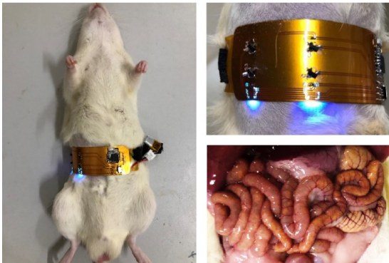
Supplementary Figure 5 The LED device mainly irradiates the small intestine of rats with its GLP-1 higher absorption capacity.
