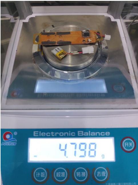
Supplementary Figure 4 The weight of the battery attached to the LEDs is 4.798 g.
