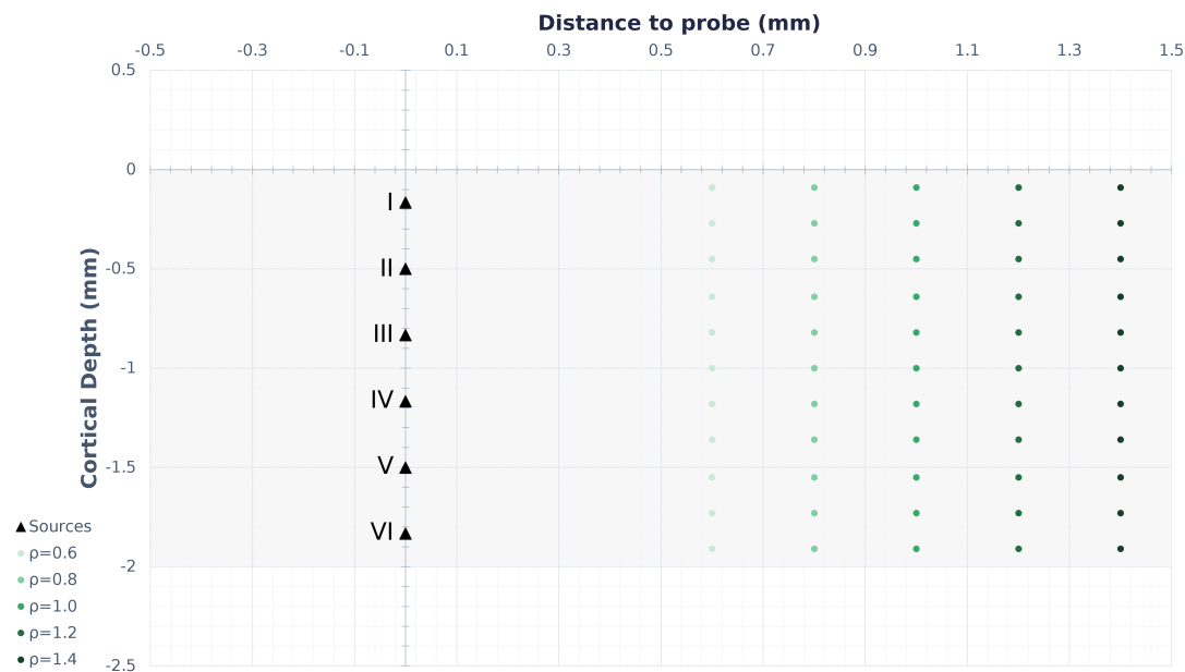
Figure E1. Schematic of the locations of the sources in every layer and the probe contacts for the different distances to probe ( \rho ) in the grey matter (2 mm).
