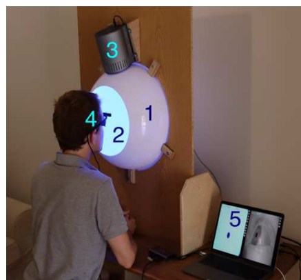
144 Figure 2. Stimulation and measurement system: 1) integrating sphere constructed from two acrylic 145 half-domes, housed and stabilized with a wooden fixing plate, 2) inside coating of Avian-B high 146 reflectance paint to scatter light homogenously, 3) STLAB light source mounted above entry port, 4) 147 Pupil Core eye-tracking headset, and 5) laptop running Pupil Capture and custom Python software. 148 The photograph was taken with the participant's permission.
