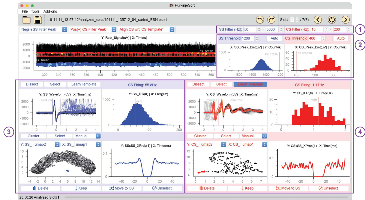
Fig. 3. Main window of P-sort. 1. Specification of filter properties for the AP and LFP channels. 2. Threshold selection and the distribution of voltage peaks for events detected in the LFP and AP channels. 3. Identification of simple spikes. The windows include spike waveforms aligned to peak voltage, distribution of instantaneous firing frequency, conditional probability \Pr(S(t)|S(0)) demonstrating a suppression period, and clustering using UMAP. 4. Identification of complex spikes. The windows include spike waveforms aligned to a learned template (yellow), distribution of instantaneous firing frequency, conditional probability \Pr(S(t)|C(0)) demonstrating suppression of simple spikes, and clustering using UMAP. The red traces indicate complex spikes that have been distorted because of nearby simple spikes.
