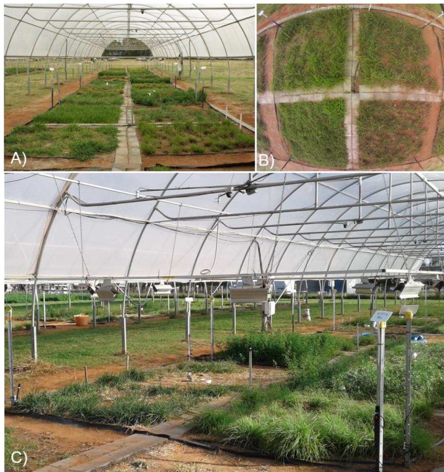
Figure 2. The Pastures and Climate Extremes (PACE) field facility located at Western Sydney University in Richmond, New South Wales, Australia. A) There are six open-sided polytunnels, each with eight experimental plots; B) Experimental plots (4 x 4 m) received a drought, warming, or drought + warming treatment and are each divided into four discrete 2 x 2 m subplots comprising nine different pasture species in monoculture; C) Heater (infra-red: IR) arrays were mounted above the vegetation canopy and warmed the plot surface an average of 3 °C above paired (control, drought) ambient temperature plots.
