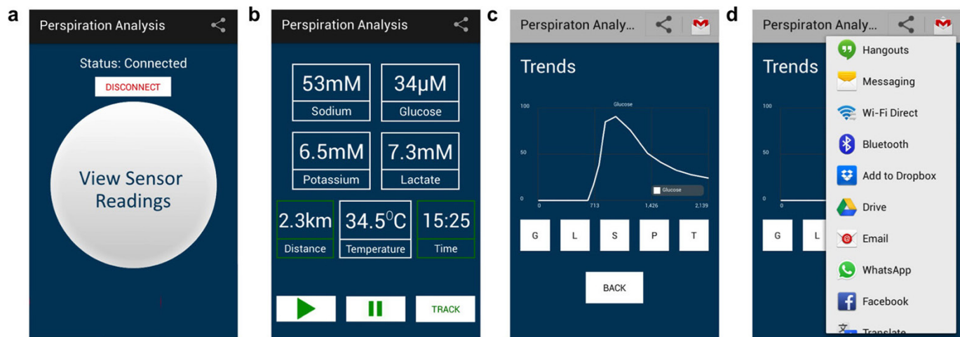
Extended Data Figure 3 | The custom-developed mobile application for data display and aggregation. a, The home page of the application after Bluetooth pairing. b, Real-time data display of sweat analyte levels as well as skin temperature during exercise. c, Real-time data progression of individual sensor. d, Available data sharing and uploading options.
