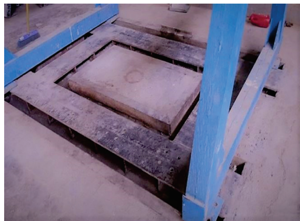
Fig. 3 Strong floor constructed for the experiments
