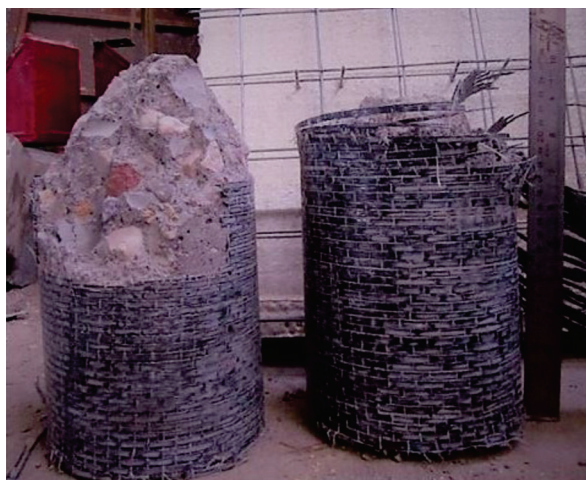
Fig. 6 Rupturing of the CFRP wrapping
